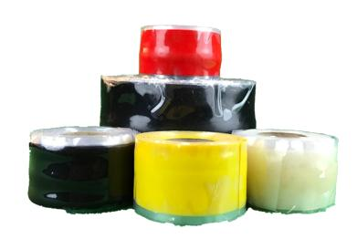
DIRECTIONS FOR USE: 1) Wrap NEX TAPE around project by stretching and overlapping onto itself. Stretch at least double to ensure a good bond, for high pressure leaks stretch to maximum amount. The tighter the tape is wrapped, the quicker and stronger the bond. 2) Continue wrapping the tape around project by overlapping 50% onto itself so that ½ the width is covered. NEX TAPE works on either side. Additional tape can be applied over project at any time in the future.
